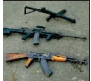
From the top, Sterling 9 mm sub-machine gun, Sterling 5.56 light machine gun and an AK47.
